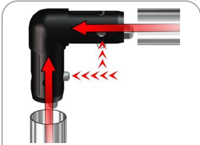
Assemble frame corners using TC-30-90. Label codes will be on backside of tube. It is best to assemble frame laying flat.
