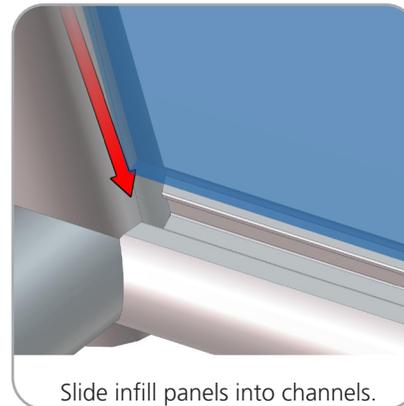
Slide infill panels into channels.
