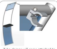
Tube clamps will come attached to frame. Position accent in front of backwall in desired location.
