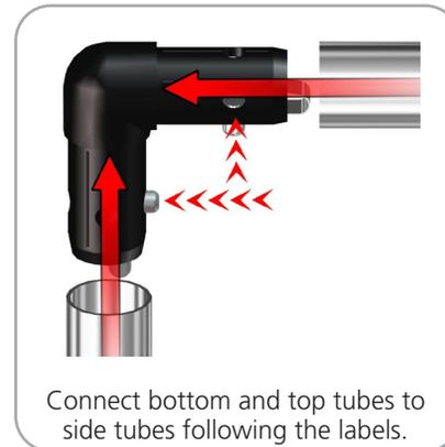
Connect bottom and top tubes to side tubes following the labels.
