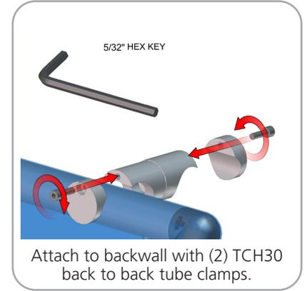
Attach to backwall with (2) TCH30 back to back tube clamps.
