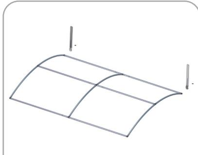
Attach feet with Allen key. See next step for detailed view.
