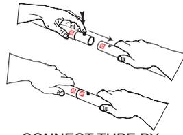
CONNECT TUBE BY PRESSING PUSH PIN BUTTON AND SLIDE OVER
