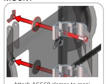
Attach ACC60 clamps to monitor mount with a bolt and washer, tighten with wingnut.
