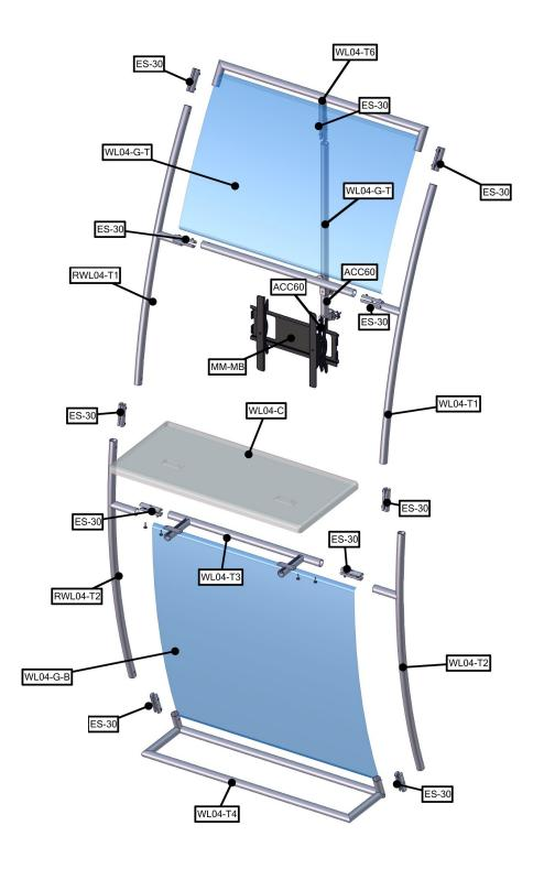
WL04 Frame Assembly: Assemble unit by laying tubes flat on the floor. Connect the tube rails following the labels by matching number to number. See detailed drawing.
