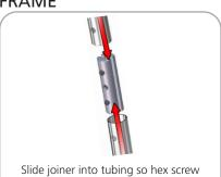
Slide joiner into tubing so hex screw sits in the hole on tubinger. Tighen hex screw so the joiner separates & tightens against the inside of the tubing, locking the joiner and tubing together.
